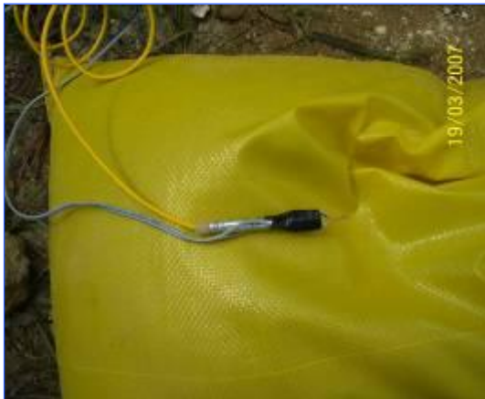
Detonator with attached bell wire.
